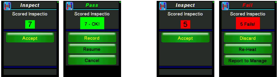
Figure 31: Two inspection examples (Left) Inspection score passed. Press Record to continue. (Right) Inspection score failed. A screen follows with corrective actions.
