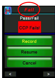
Figure 30: Sample Fail CCP screen followed by screen with listing corrective actions.
